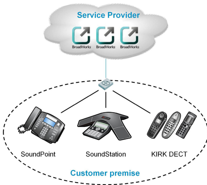
Figure 1: Hosted voice communication services using BroadSoft and Polycom equipment
